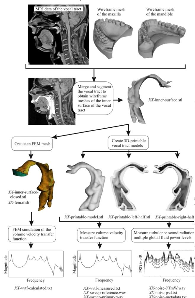
**Figure 1:** Overview of the data acquisition and processing. The shown images and spectra are for the tense vowel /e:/ of speaker 1. XX in the file names is a placeholder for the speech sound labels.
