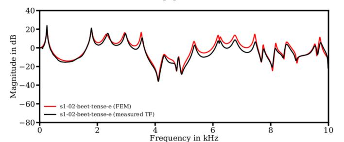
**Figure 2:** Experimentally and numerically determined volume velocity transfer function for the tense vowel /e:/ of speaker 1.
